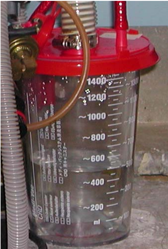
Figure 5.4 An example of a vacuum canister with inner “liner” used to collect effluent
